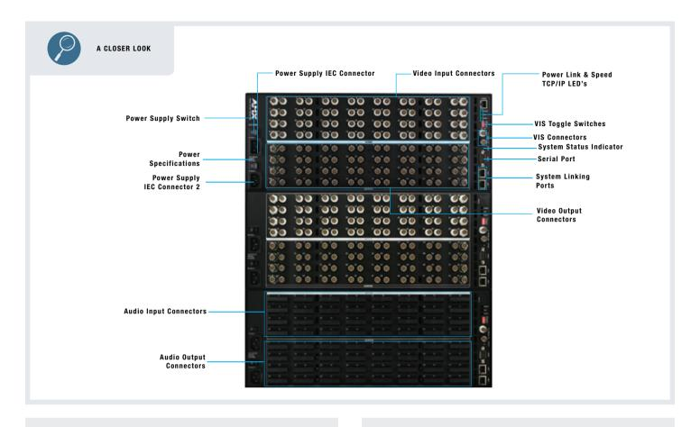
System is made up of 2 standard video enclosures and 1 stereo audio enclosure  $\,$
