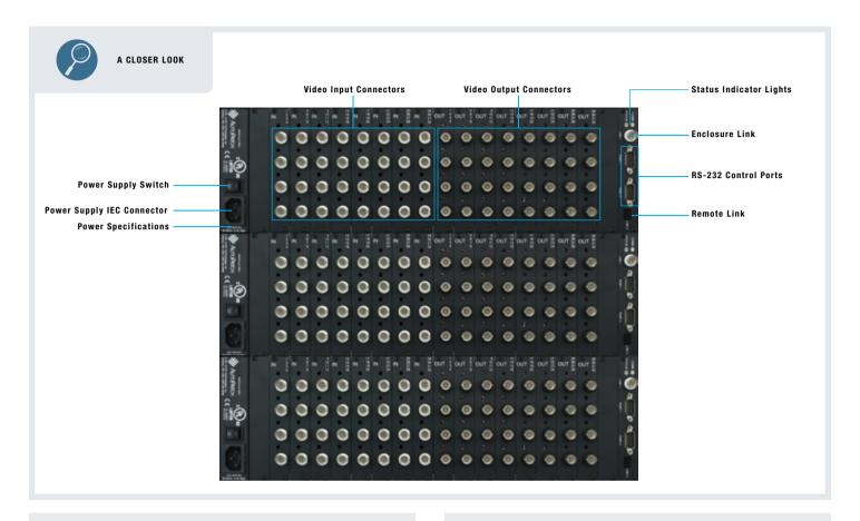
HDTV/Component systems are made up of multiple 3 RU enclosures
