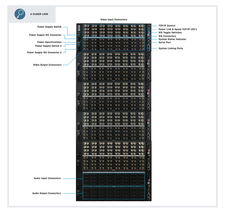
RGBHV with stereo systems are made up of 3 ultra-wideband video enclosures, 2 sync enclosures and 1 stereo audio enclosure
