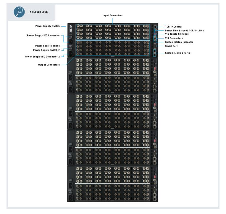
This system is made up of 3 ultra-wideband video enclosures and 2 sync enclosures. It occupies 20 RU. Specifications listed below are for individual enclosures.
