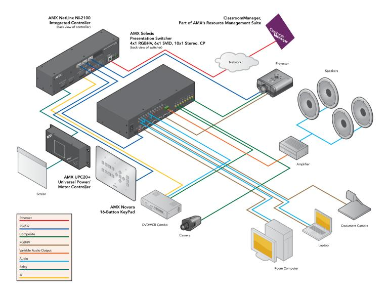
projector or display the switcher is feeding video to and in some entry level applications this eliminates the need for a central controller. The switcher's small form factor, flexible mounting options and simple to use setup software, reduces installation time, centralizes the room's video and audio switching and simplifies operations.
